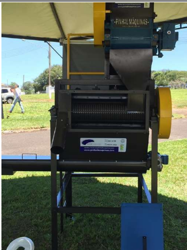
Figure 11: Machado Campus technological innovation of a coffee pulper with zero water consumption .
